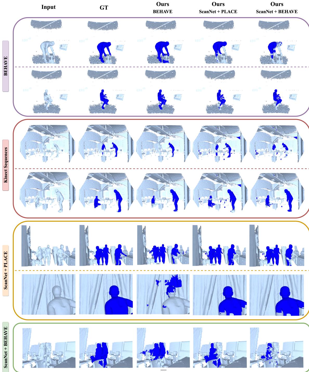
Figure 3. Example predictions and comparisons. From left to right, we show: (1) input point cloud, (2) ground truth segmentation, result from (3) model trained with the BEHAVE dataset, (4) model trained with depth scans from ScanNet scenes populated with PLACE, (5) model trained with depth scans from scenes populated with BEHAVE, using two labels person and background . Each box denotes results on a different dataset: BEHAVE , Kinect RGB-D Sequences , ScanNet+PLACE and ScanNet+BEHAVE . We demonstrate successful results on challenging scenes with one or more humans, often occluded and closely interacting with their surroundings. Bottom two rows demonstrate failure cases for different methods: first one is a close-up view of a human. While models trained with ScanNet+PLACE and ScanNet+BEHAVE perform well on this point cloud, the model trained with BEHAVE fails, whose training only involves humans with fully visible bodies. Last row demonstrates a scene with very noisy human bodies, which is challenging for our models to handle.
